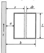
(a) At an instant when the current is i, find the magnitude of the magnetic field B(r) at a distance r in terms of i and r.
